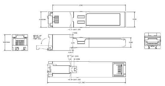
Figure 2. SFP24-(G)T mechanical dimensions
